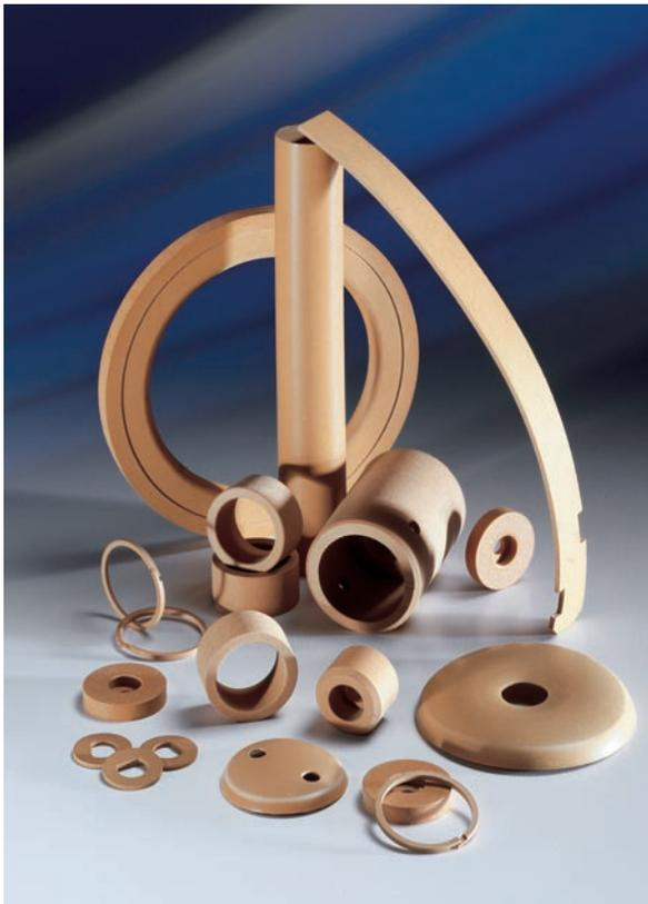
Rulon® J is an all-polymeric reinforced, dull gold colored PTFE compound that operates exceptionally well against soft mating surfaces such as 316 stainless steel, aluminum, mild steel, brass and other plastics. The unique "shaft friendly" material is also low in friction and wear and self-lubricating.
